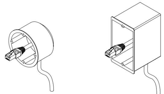
3. Connect the ethernet cable to the Wall-S1 unit.
