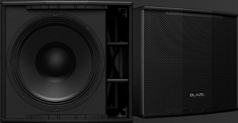
Designed primarily for free-standing installations, the BL18S features an 18-inch bass driver housed in a reflex-loaded enclosure, delivering low-frequency bandwidth down to 31Hz at -10dB, with maximum sound pressure levels reaching 136dB at 1m. Multiple BL18S subwoofers can be installed in stacked pairs and configured via amplifier presets to deliver either omnidirectional or cardioid directivity characteristics, ensuring exceptional sound distribution.
