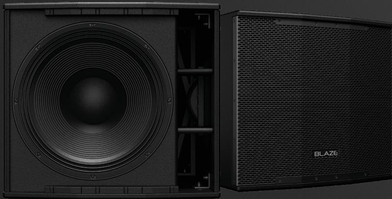
Designed primarily for free-standing installations, the BL18S features an 18-inch bass driver housed in a reflex-loaded enclosure, delivering low-frequency bandwidth down to 31Hz at -10dB, with maximum sound pressure levels reaching 136dB at 1m. Multiple BL18S subwoofers can be installed in stacked pairs and configured via amplifier presets to deliver either omnidirectional or cardioid directivity characteristics, ensuring exceptional sound distribution.
