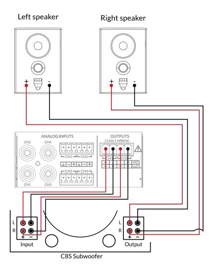
**2.** Connect L red (+) from the subwoofer output terminal to the red (+) input on your left speaker, and L black (-) from the subwoofer output terminal to the black (-) terminal on your left speaker. Likewise, connect R red (+) on the subwoofer output terminal to the red (+) input on your right speaker, and R black (-) from the subwoofer output terminal to the black (-) terminal on your right speaker.
