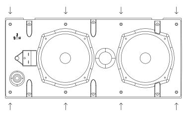
Turn the tweeter counter-clockwise to remove it from the baffle. Reinstall the new tweeter by pressing it towards the horn section of the baffle and turn it clock wise until you hear a "click".
