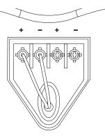
Connect the red (+) and black (-) speaker cable to the left + and right - screw terminals. Use the right + - terminals to link to another speaker.
