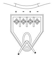
If you use the sliders, you can mount the speaker cables to the terminal at this point. If you use the mounting points, it is easier to install the speaker first and mount the cable to the terminal after the speaker is mounted to the wall.
