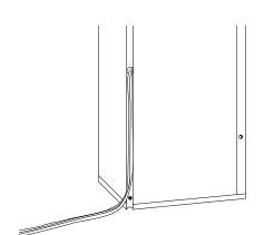
③ Run the speaker cable through the tube positioned at the rear of the cabinet to the terminal at the front baffle.
