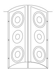
Likewise, three cabinets can be mounted together to cover 270 degrees around a free-standing corner. Simply couple three cabinets together using 9x3 mm bolts and mount the speakers to the corner with the integrated mounting points.
