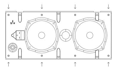
Turn the tweeter counter-clockwise to remove it from the baffle. Reinstall the new tweeter by pressing it towards the horn section of the baffle and turn it clock wise until you hear a "click".
