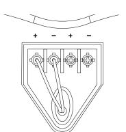
Connect the red (+) and black (-) speaker cable to the left + and right - screw terminals. Use the right + - terminals to link to another speaker.
