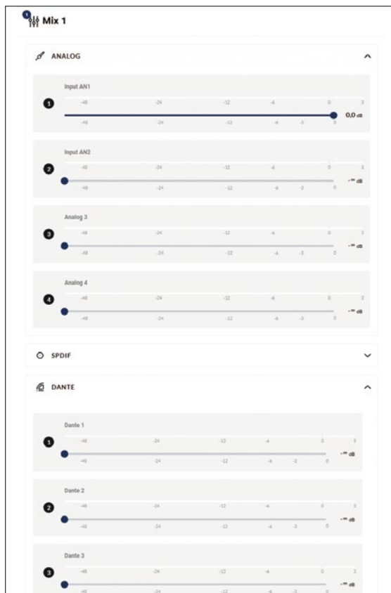
Fig. 3: One of a total of four mixers in the DSP, with which the signals for the zones can be freely compiled from all inputs
